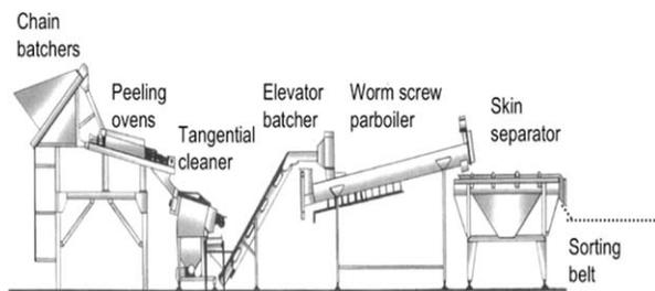
**FIG. 1.** SCHEMATIC DIAGRAM OF A BRULAGE CHESTNUT PEELING LINE (BOEMA; NEIVE, ITALY)
