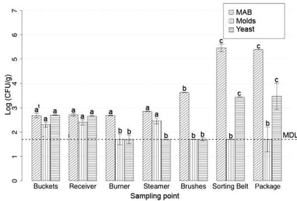
**FIG. 3.** TOTAL MAB, MOLDS AND YEAST COUNTS (LOG CFU G<sup>-1</sup>) ON PEELED CHESTNUT SAMPLES (BRULAGE PEELER – BOEMA; NEIVE, ITALY) <sup>1</sup>Values followed by the same letter within organisms are not significantly different at  $P < 0.05$  (ANOVA) (Tukey multiple comparison of means). Minimum detectable level (MDL), represented by a dotted horizontal line = Minimum possible count (0.5) x minimum dilution factor x inoculated aliquot (100  $\mu$ L). Error bars indicate standard deviation.
