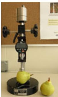
**Q.** Could someone at UC Davis tell me if in your experience a Durometer gives more consistent readings if used on a motorized stand? In other words, if the durometer tip is contacting the fruit at a steady rate of speed and direction, does this give more reliable readings than using it "hand held"? (K.A.J.)
