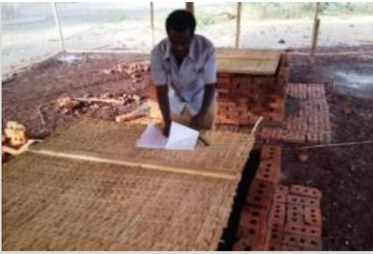
Measuring relative humidity and temperature inside the Zero Energy Cooling Chamber (ZECC) using digital thermo-hygrometer at Samara Agricultural Research Center of Ethiopia. The average differences in dry bulb temperature between ambient and inside the ZECC were 15.34 °C, with the average difference in relative humidity of 56.6% during the 30 days of storage of tomato fruits.
