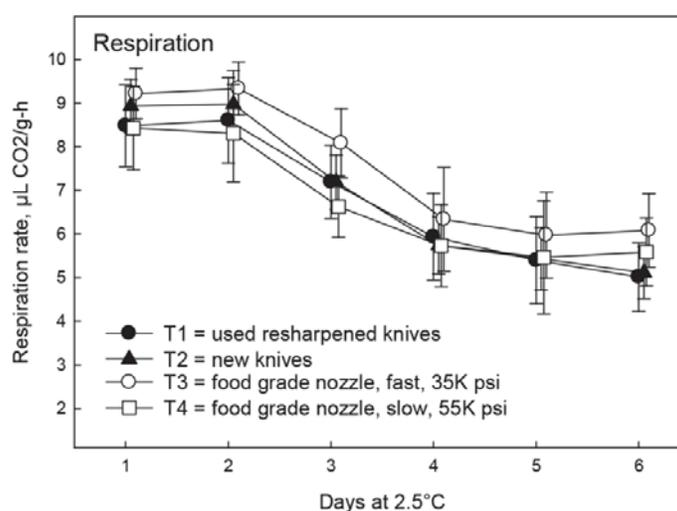
Figure 2. Respiration rates of salad-cut romaine ‘Sun Valley’ prepared by stainless steel blades or by food-grade waterjet nozzles and stored in air at 2.5°C. Data are means of four replicates ± standard deviation.
