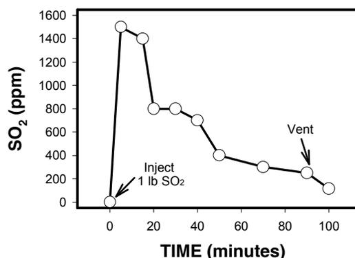
Fig. 1. Sulfur dioxide concentrations measured with Kitagawa tubes in a 2.377 ft<sup>3</sup> marine container after fumigation with one pound of gas.
