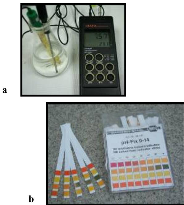
Fig. 3. Portable electronic pH meter (a) and color-changing paper indicator (b) for fast measurement of water pH.
