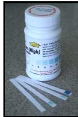
Fig. 4. High range test strips for measuring available/free chlorine in the water are a practical way to monitor dosage. In combination with pH measurement, optimal active/effective chlorine (hypochlorous acid) will be present when pH is near 7.0.
